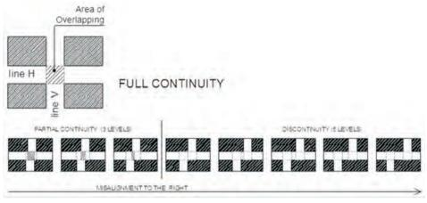
Figure 3: levels of misalignment of a generic intersection
